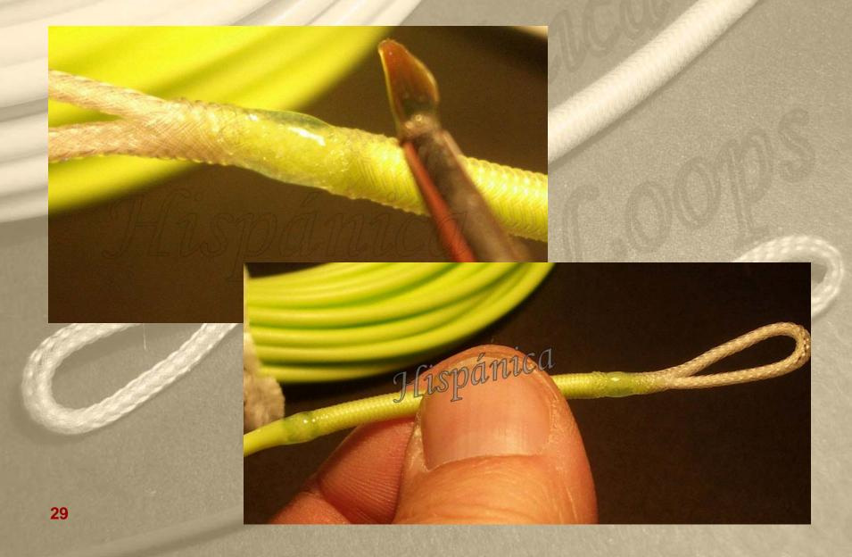
• STEP 23: TIP LOOP. Build a braid loop like the previous one. Now there's no need to reinforce passing the line core through it, as this area won't be subjected to so much mechanical effort during cast. Just make a sharpen cut on the tip to facilitate penetration and thread it up to the start of the loop, making sure that the inside braid doesn't shrink.
