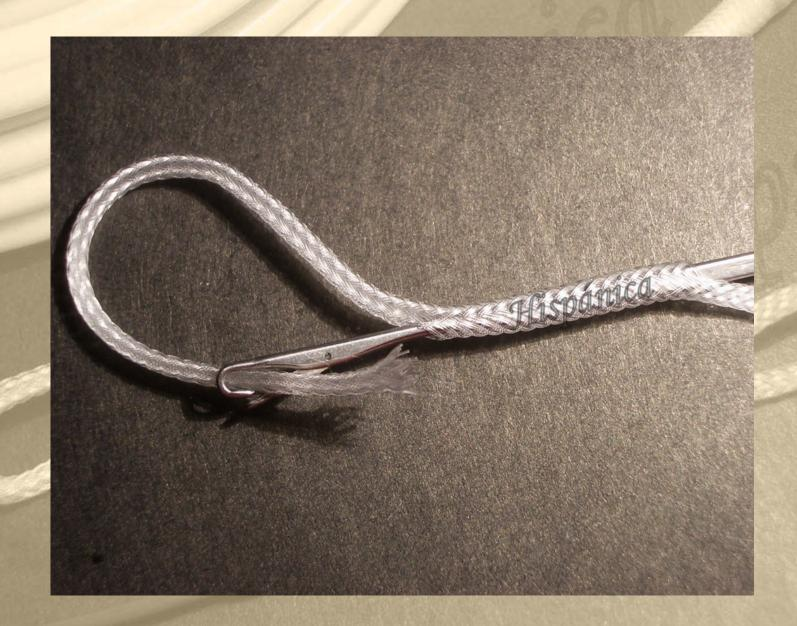
• STEP 8: Go back with the needle to pull out the end of the braid.
